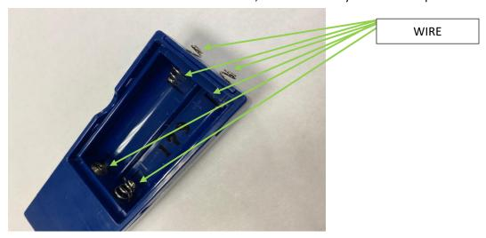
**Step 4:** Inspect the two round gold contacts inside the manikin as shown for corrosion.
