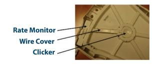
Remove the Wire Cover and disconnect the Rate Monitor from the Clicker.
