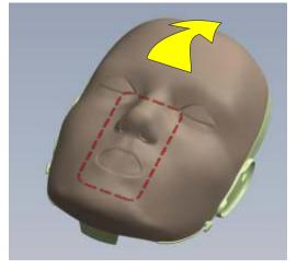
4.) Attach face skin assembly from step 3 to face ensuring that the Oral/Nasal insert is aligned with the opening in the face. Seat the assembly by pressing down along the red dotted line shown here. Confirm outer edges of Face Skin are secure by running your thumbs from the brow of the face to the crown of the head using gentle pressure to slightly stretch the skin over the face.
